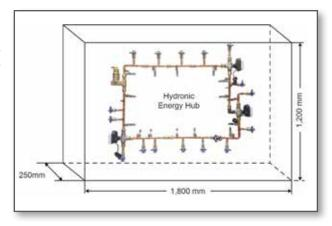
The Hub is connected using 20mm unions located at the top and bottom of the back panel. We suggest mounting the Hub in a plant room or garage on the wall or ceiling or on an external wall. If boxing-in the Hub with joinery, access through a removable cover should be considered for maintenance.
