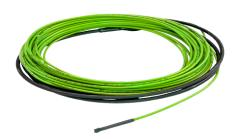
The Xcable CF, a single conducting electric cable, double insulated with PET foil and PEX layer, features an earth screen of drain-wires and aluminum foil embedded in a PVC sheath. Although the CF cables were designed for freezer applications, they may also be used for in-screed floor heating. The cables come in bulk, but can be terminated for specific lengths. The CF cables comply with IEC 60800:2009.
