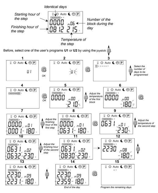
To program the remaining days, repeat step « 4 » to « 14 » and this for all the days of the week. Once you have run through the whole programming, set the thermostat in the Auto mode.
