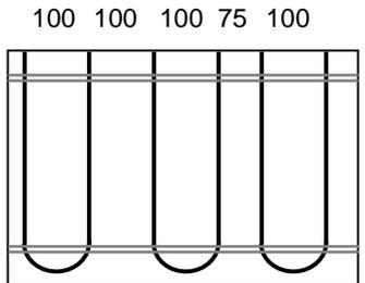
**Step 4** Nail devifast fixing strips to floor with no more than 700mm between strips
