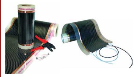
Comfortline Ceiling Foils are a radiant ceiling heating system. The foils have thin carbon heating elements sandwiched between two layers of transparent high temperature plastic laminate.
