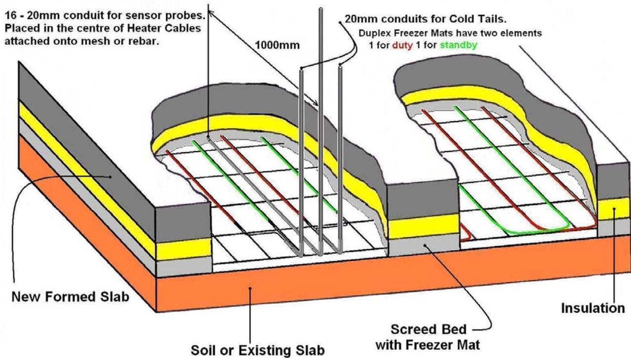
At no point in the installation should heating cables be allowed to become embedded in the thermal insulation.
