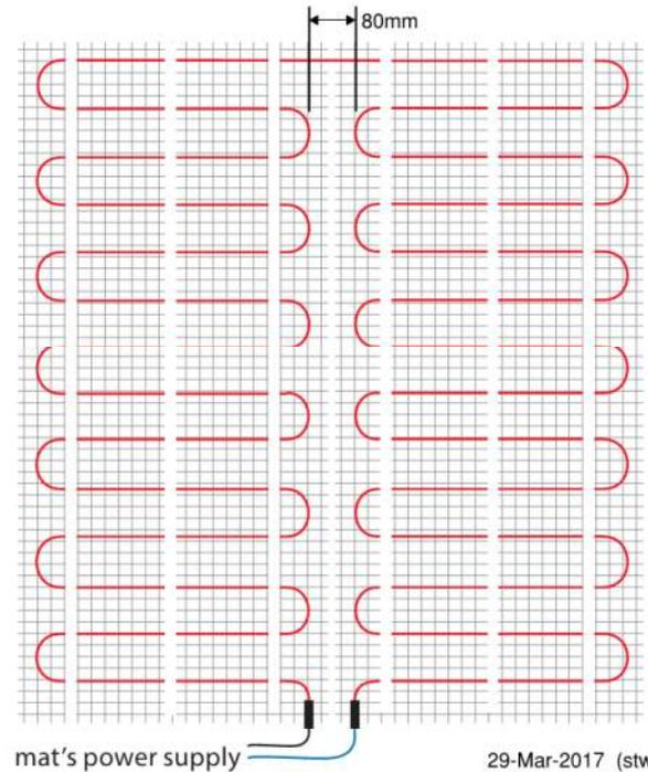
EXAMPLES of a **simple heating layout** where the mat is cut and then run next to the first mat but back the other way, keeping the sticky side down to the floor.
