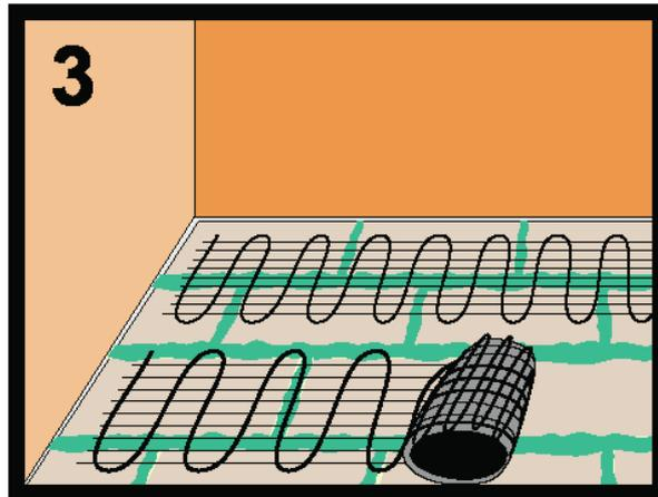
A waterproof membrane is recommended but this can be placed below or above the F-Board. The membrane must not be placed over the heating cables. The F-Board need not be protected with additional hydroinsulation.
