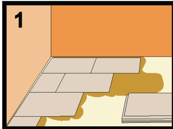
Spread the adhesive sealing cement with a notched spreader on the cement base. Place the boards as shown in Picture 1, setting and aligning them properly. Allow the adhesive material to harden, as described in the instructions for use. When laying the boards, the adhesive material must not come into the spaces between the boards. The expansion joints in the foundation must be preserved.
