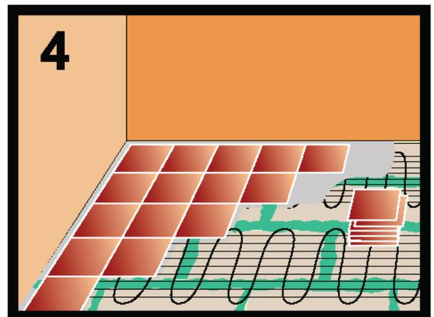
We recommend **Davco SMP Evo** cement-based flexible tile adhesive to glue down the F-Board sheets and to glue down any floor tiles to the F-Board sheets.
