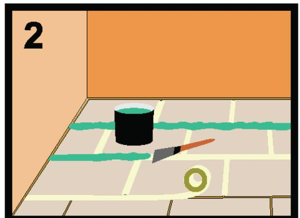
Any gaps or voids between F-Boards should be covered with reinforcing gauze fabric tape. Apply SMP Evo (or similar) adhesive material, place the tape, and spread the material over the tape with a spreader. The tape should overlap at least 20mm.
