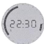
The picture at left illustrates the appearance for a Timer setting of COMFORT Heat from 6.00am to 7:30am and later from 15:30pm to 22:30pm on Day 1
