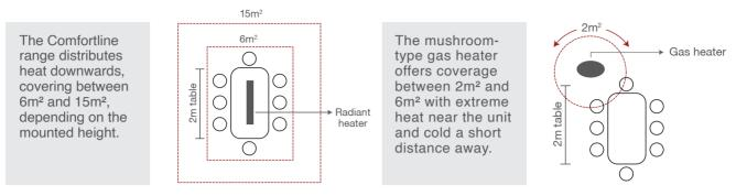
A single high capacity Comfortline panel costs about 60c/hour\* to run, while a typical mushroom heater on bottled gas can cost up to five times at \$3.00/hour\*\*.
